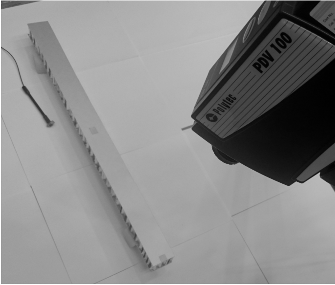
Figure 4.5: Experimental setup with a 30 mm aluminium sandwich beam supported on foam pads, excited by impact hammer and the velocity response measured by means of a laser vibrometer [1].
